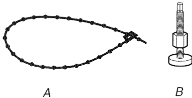
A. Beaded tie strap B. Front leveling feet with nuts (2)
