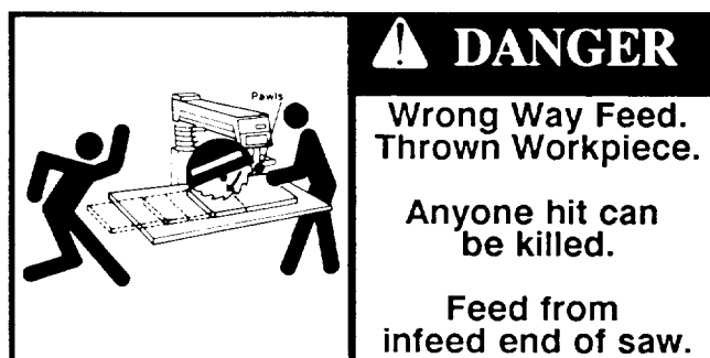
Fig. 109 Wrong Way Feed Safety Signs
