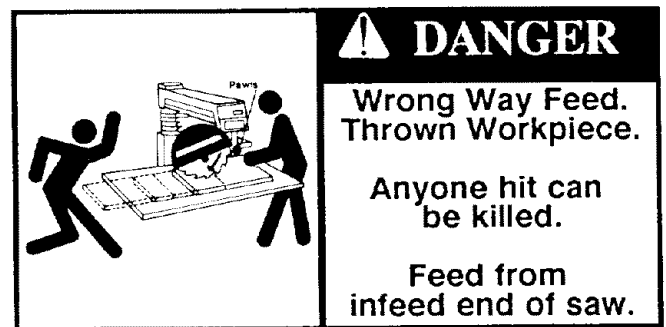
Fig. 153 Wrong Way Feed Safety Signs
