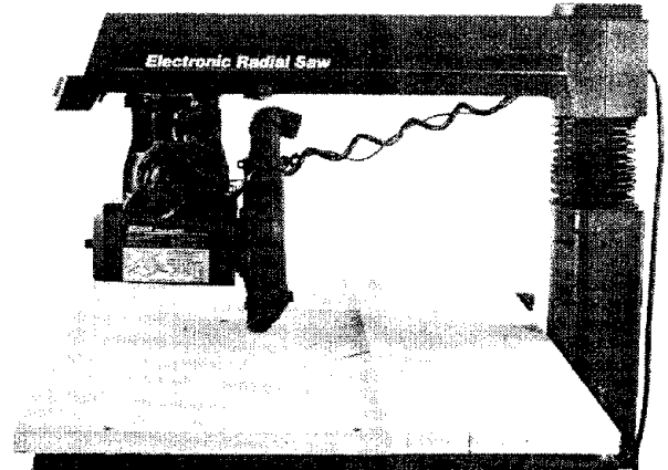
Fig. 155 In-Rip Saw Position
